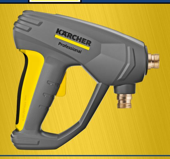
The revolutionary concept of the EASY!Force high-pressure gun ensures fatigueless working over long periods. The recoil force of the high-pressure jet is used to reduce the holding force for the operator to zero. In terms of durability, the high-pressure gun impresses with high-quality materials: the ball and sealing seat of the ceramic valve are far harder than any conceivable foreign particle. The full ceramic valve ensures a 5 times longer lifetime in comparison to other high-pressure guns.
